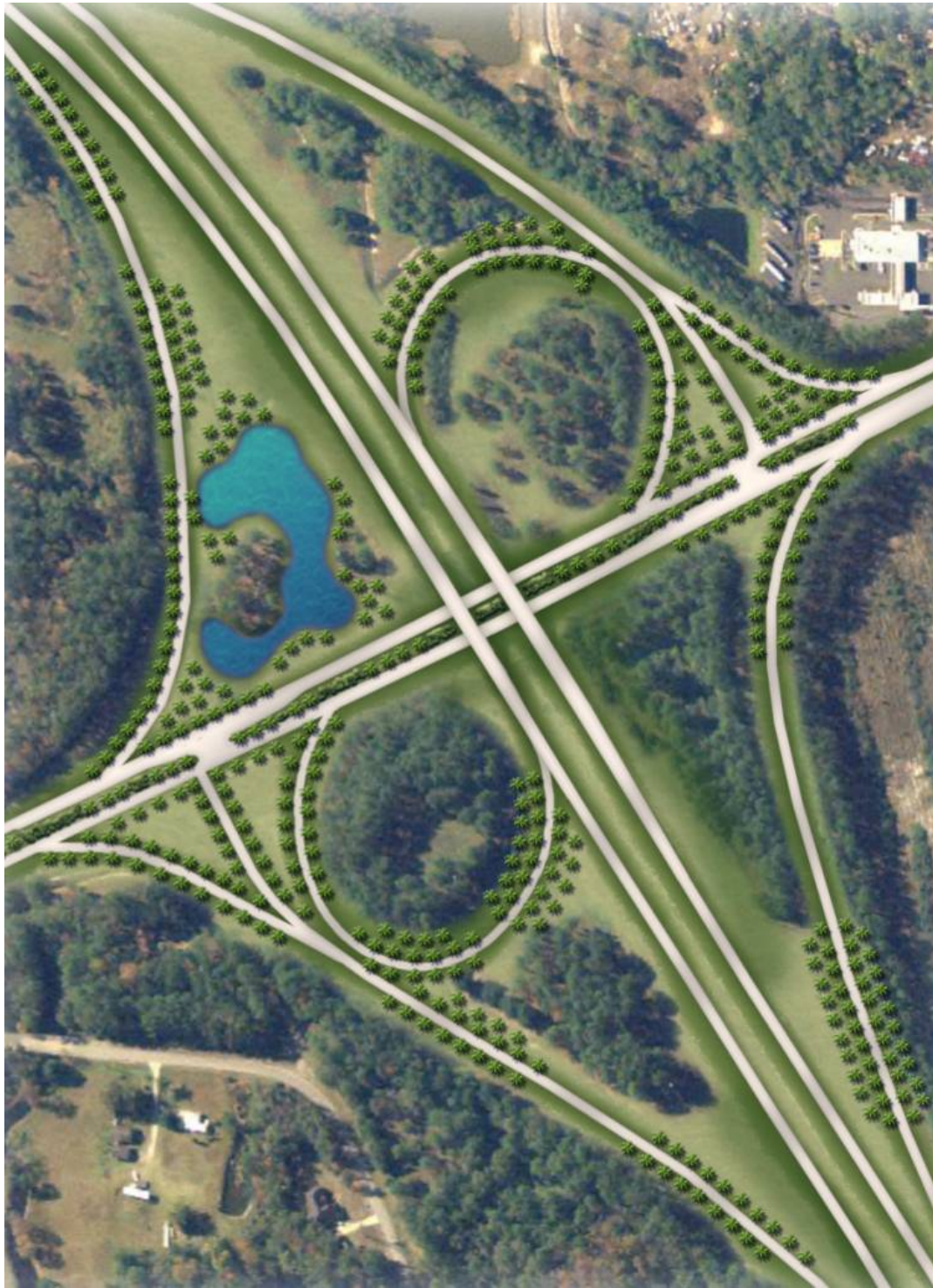
Figure 1. – Gateway Interchange – New Kings Road Master Plan
